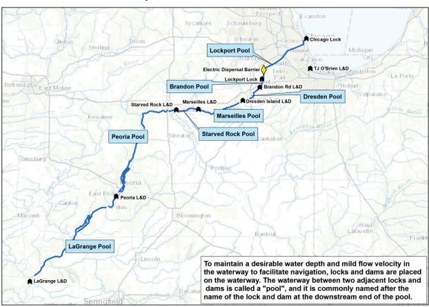
The current Electric Dispersal Barrier System, located approximately 5 mimi upstream of the Lockport Lock and Dam, is assumed to continue operation through  $T_{50}$ .
