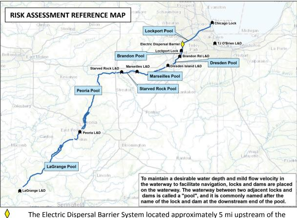
The Electric Dispersal Barrier System located approximately 5 mi upstream of the Lockport Lock and Dam is assumed to continue operation through  $T_{50}$ .
