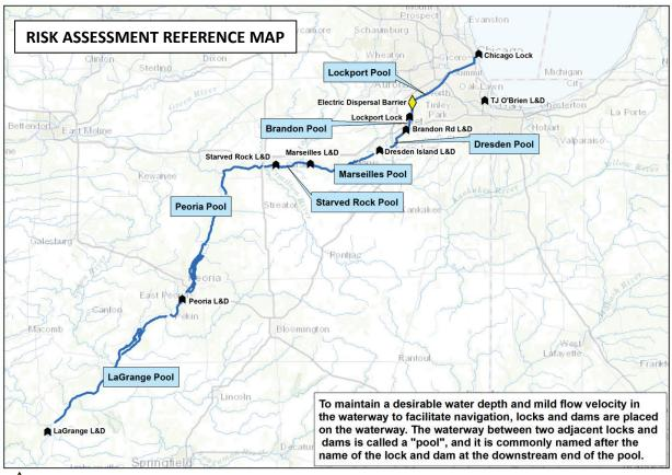
$\diamond$  The Electric Dispersal Barrier System located approximately 5 mi upstream of the Lockport Lock and Dam is assumed to continue operation through T<sub>50</sub>.
